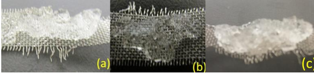
Figure 5.5 – Visual Appearance of Treated Hydrogels: (a) untreated hydrogel, (b) hydrogel treated with dry scCO 2 , (c) hydrogel treated with presaturated scCO 2
